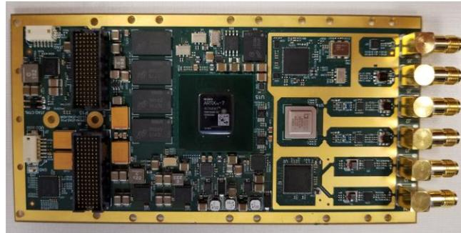
The XA-500M is an XMC IO module featuring two 14-bit, 500 MSPS A/D channels and two 16-bit, 615 MSPS DAC channels designed for high speed stimulus-response, ultrasound, and servo control applications.
